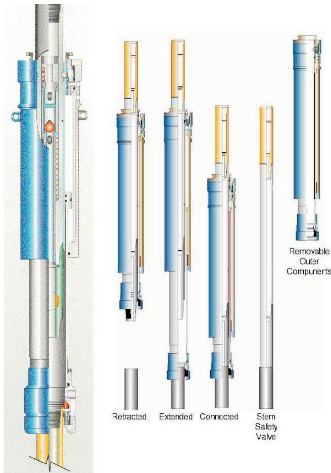
Figure 1: CFT allows normal pipe-handling operations to be conducted as if the unit were not installed. Seal prevents mud spillage on the rig floor.
