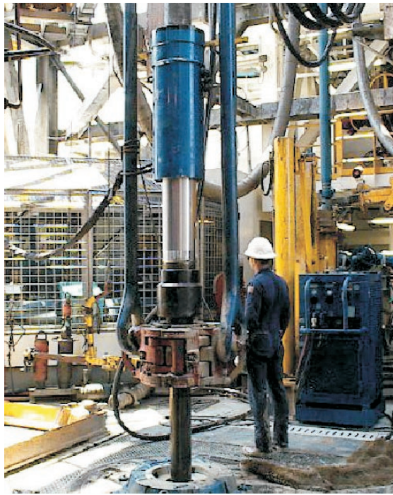
The OES circulating/flowback tool can allow pipe to be run or pulled faster while avoiding the loss of expensive drilling mud.
