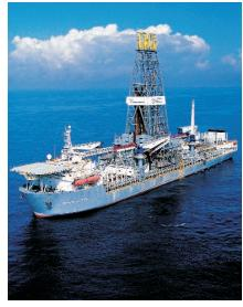
Discoverer Enterprise is fitted with dual activity system, can drill in 10,000 ft water depths.
