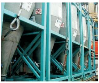
The number of ISO- The number of ISO-Pumps located on the rig for interim storage of drill cuttings will vary depending on rig characteristics and logistics.
