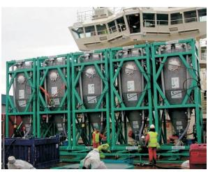
The same number of ISO-Pumps are usually installed on the boat wide as a standard con- as on the rig. Material is moved from rig to boat with flexible hose.
