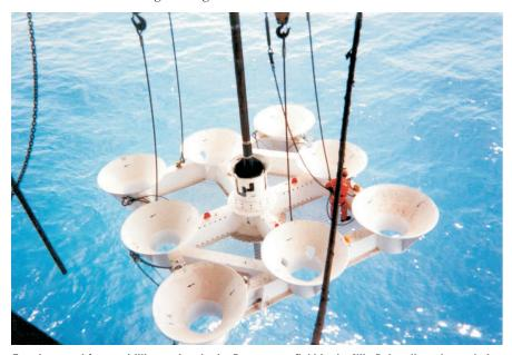
Template used for pre-drilling project in the Rosetta gas field in the Nile Delta allowed completion of project in time to meet gas delivery dates. 4 wells were pre-drilled and 2 30-in. conductors set.
