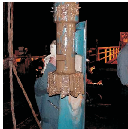
An 11 3/4-in. OD liner was installed through a whipstock window cut in the 13 5/8-in. casing.
