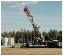
Versatile new rig design can be used from vertical to slant in a variety of drilling operations.
