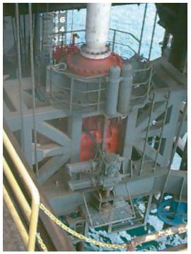
Surface BOP technology has been used successfully by A report of each break-out ses-Unocal in Southeast Asia utilizing Transocean's Sedco 601 semisubmersible. The technology enables the rig to work in deeper waters.
