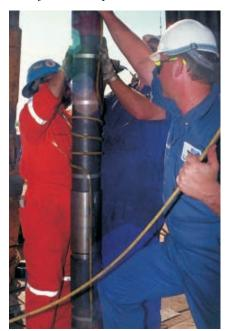
Baker Oil Tools technicians make up the world's first downhole electric wet disconnect tool.
