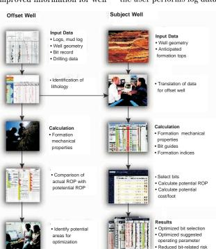
Following a software-driven bit selection process when selecting the optimum bit series for a new well allows more accurate translation of offset mation mechanical properties data to the planned well and more comprehensive cost/risk/performance analysis of the wide range of bits.
