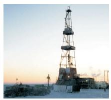
This modular Russian rig can be skidded from site to site, rigged up, wells drilled and completed and demobilized in one winter season.
