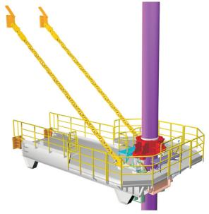
Atwood Oceanics will present a 500,000 lb motion compensated conductor tension system (CTS) that will be installed below the cantilever substructure on the 400 ft water depth jackup Atwood Beacon
