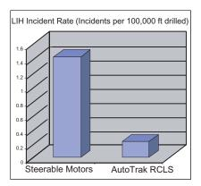
Continuous pipe rotation, smoother trajectory and overall improved hole gauge quality reduce stuck pipe and lost in hole (LIH) incidents.
