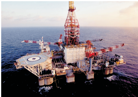
BP installed polyester mooring in a taut anchoring system on Diamond Offshore's Ocean Confidence in the Gulf of Mexico.
