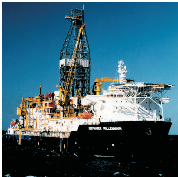
The Deepwater Millennium, one of the first of the ultra-deepwater newbuilds, is of the Pathfinder Class of vessels rated for 10,000 ft of water.
