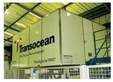
Transocean's new state-of-the-art marine simulator uses computer-controlled linear-actuator motors rather than hydraulics to replicate up to 15 degrees combined pitch and roll.
