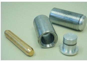
The components of the VDBP system. The new plug has one O-ring with a backup ring in an external groove on the plug. The O-ring seats inside a speciallybuilt collar threaded on the end of the tubing. Two small shear pins help hold One alternative the plug in place while running in the well.
