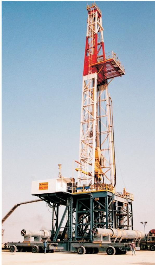
With Rig Buggies, the time required to move the rig to the next well-site, usually about 50-100m away, is about 40 hours, although there is scope for reducing this time to about 35 hours.
