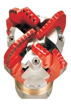
The expandable drill bit's closed configuration is shown on the left with the expanded mode on the right. During field tests with Unocal in Indonesia, weight on bit required to achieve a specificed controlled penetration rate was 39% lower than for offset tricone runs.
