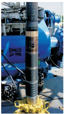
The expandable metal cladding system is deployed and expanded utilizing an innovative hydraulic piston/anchor system that allows flexibility in the length of the deployed clad from short sections to unlimited lengths, providing re-lining of casing with pressure integrity in a one-trip system. IADC/SPE 87212
