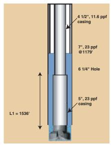
Pipe rotation plays an important role in determining ECD in the annulus between casing and a wellbore. IADC/SPE 87149
