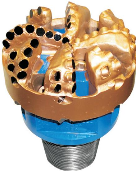
**Bit design enhancements that permit operators to break through the technical limitations set by hard formation drilling with roller cone bits include stable bit designs and advancements in thermostable cutter technology.** IADC/SPE 87098
