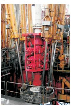
Shell Deepwater Services conducted a comprehensive risk assessment and management program with the objective of introducing surface BOP operations to a number of deepwater regions around the world. IADC/SPE 87112
