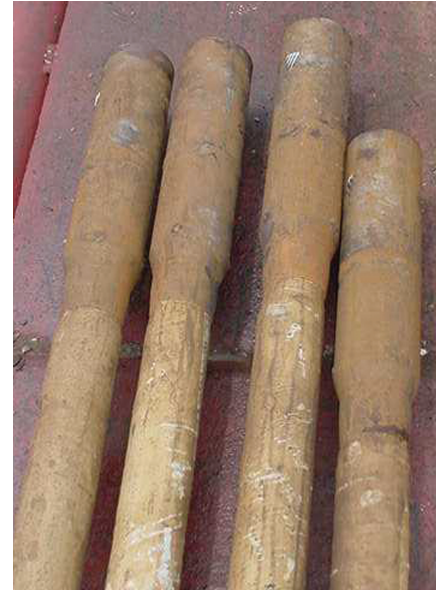
Composite pipe experienced minimal wear during testing and in-ground evaluation.
