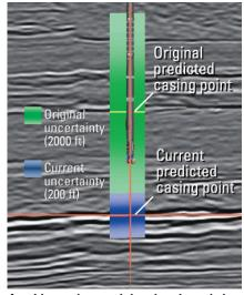
Acquiring and transmitting data in real time enables the operator and driller to reduce uncertainty ahead of the bit, potentially saving a casing string.
