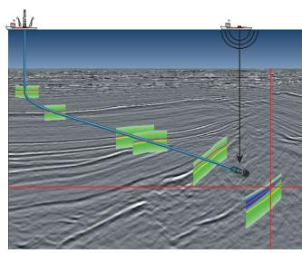
Checkshot data is used to place the bit on the seismic map to aid in navigation, select casing points and prepare for potential hazards ahead of depth uncertainty the bit sych as faults, pore pressure variations or formation variations.
