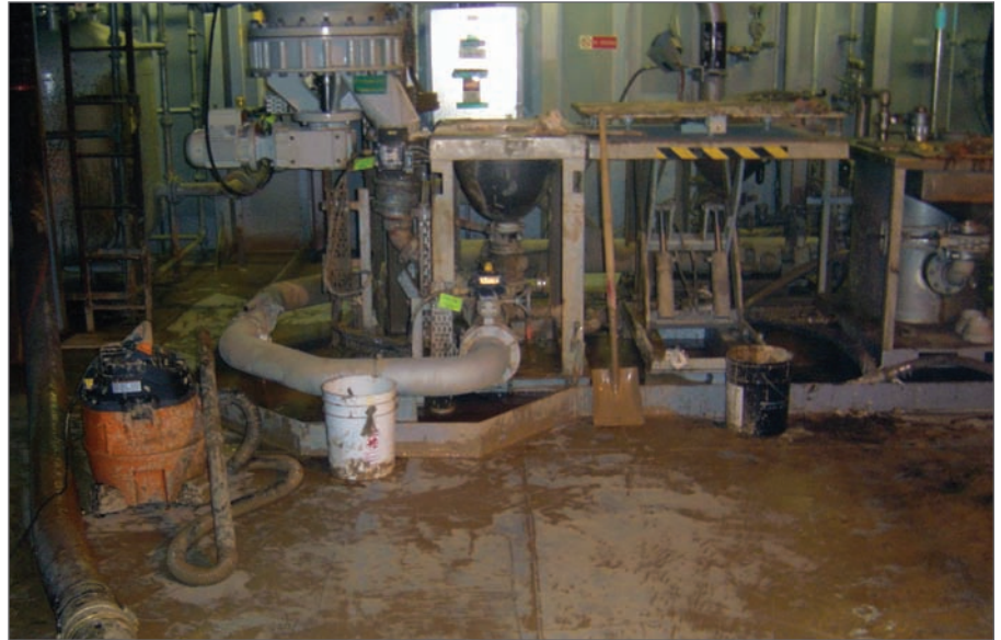
Manual mud-mixing equipment have a higher risk of imprecision in the mixing process compared with highly automated systems.
