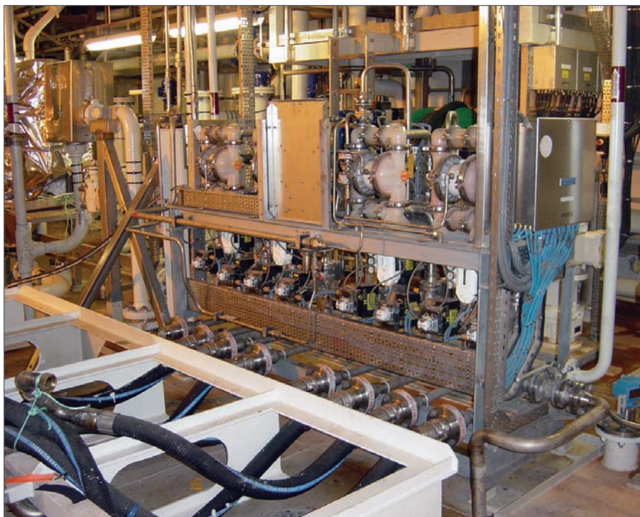
The addition of liquids is fully automated on the Valhall water-injection platform.
