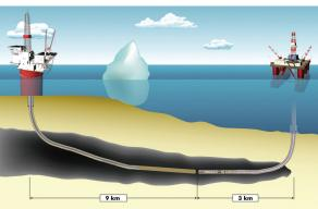
The planning and execution of what is believed to be the world's first planned successful joining of casing strings for two horizontal wells will be discussed at the conference. SPE/IADC 92685.
