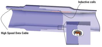
Drillstring components capable of transmitting data at rates up to 2 megabaud have these issues and provides a been developed and successfully tested in commercial drilling applications. The new forward-looking statement technology can improve well productivity and reduce drilling time. SPE/IADC 92477. hydraulics and related con-
