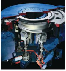
A mud pump utilizing six pistons in minimized pressure pulsations can provide a nearly constant steady flow. SPE/IADC 92507.
