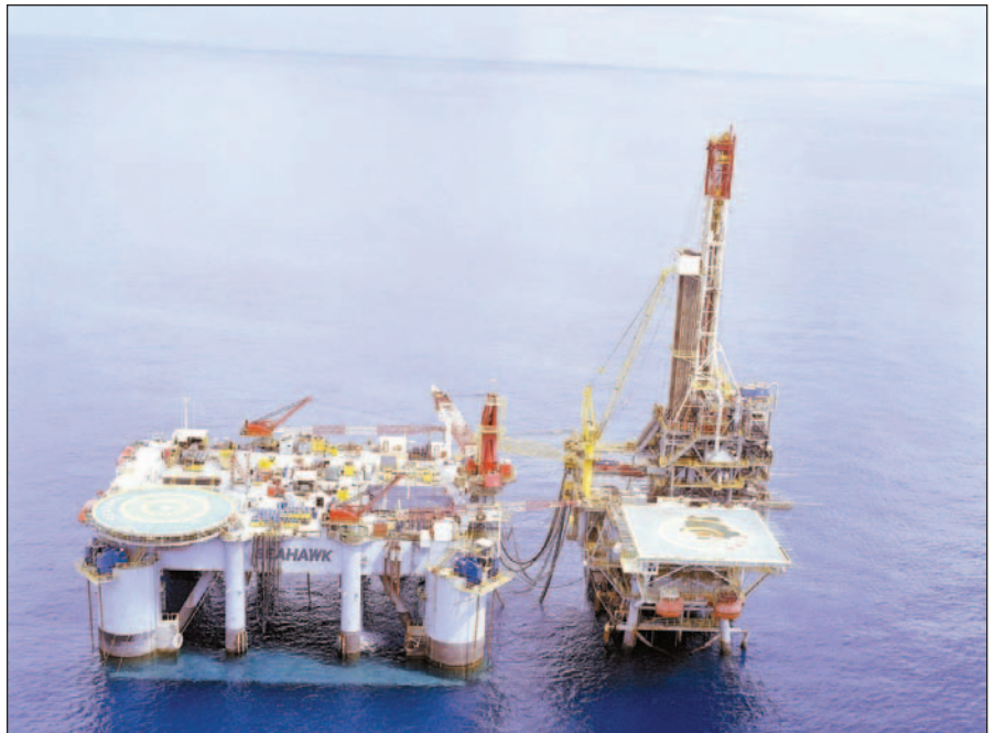
Semi tender-assist drilling units, such as the Atwood Seahawk shown above, can solve the problems of weight, space and operating efficiency found with TLPs, fixed platforms and spars, said Mark Atwood, general manager of technical for Atwood Oceanics. The Seahawk worked 14 years without a lost-time incident.
