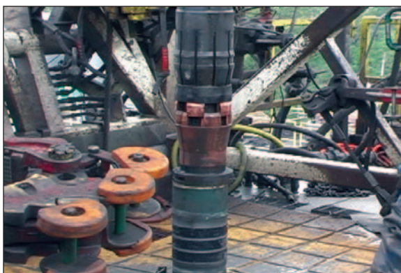
Figure 2 (above): As part of a recent Oklahoma installation, the liner was expanded 18% to 8 5 / 8 -in. nominal and 8 1 / 2 -in. drift ID. The operations was performed in 15-ft (5-m) increments by applying drill pipe pressure to the expansion tool, then de-pressuring and slacking off. Figure 3 (below): In this fashion, the entire 1,514-ft (461-m) liner was expanded, completed with a truck-mounted cement pump to supply expansion pressure.
