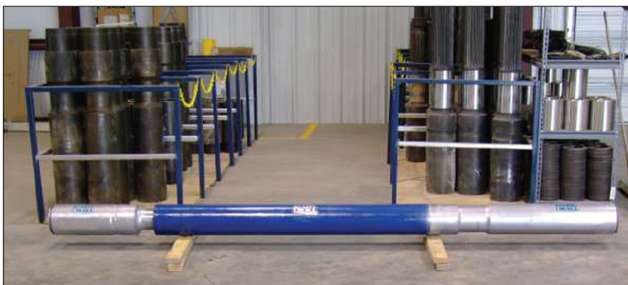
Stabil Drill's new line of shock tools can operate in temperatures of 275-450°.
