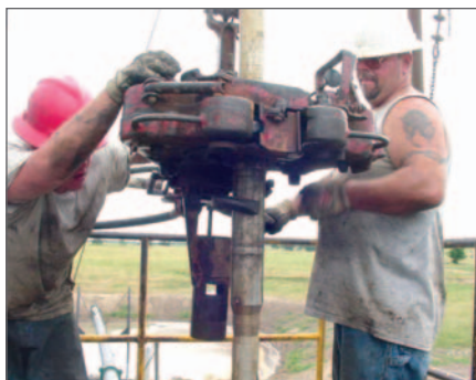
Figure 2 (above) shows short-radius drill pipe being added to the string in a field test, in which the pipe was run for more than 160,000 cycles at an average RPM of 70, air pressure 300 psi and torque of 1,000 lb-ft. After a week of drilling, the pipe showed little to no signs of wear, as seen in Figure 3 below.
