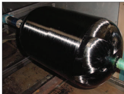
Figure 5 (above): Composite power transmission shafting, such as this single-piece composite automotive shaft and corresponding two-piece metal shaft, should find more use in oil E&P. Figure 6 (right): A graphite-overwrapped titanium pressure bottle can be a weight-saving technology applicable to pressure vessels for offshore operations.
