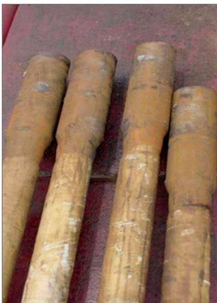
Figure 2 (above) shows short-radius drill pipe being added to the string in a field test, in which the pipe was run for more than 160,000 cycles at an average RPM of 70, air pressure 300 psi and torque of 1,000 lb-ft. After a week of drilling, the pipe showed little to no signs of wear, as seen in Figure 3 below.
