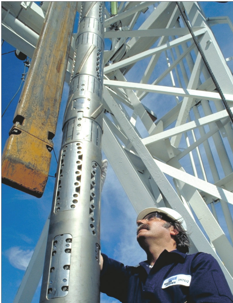
The OnTrak tool is used in Nagar #1 to provide continuous downhole annular pressure measurements to the DAPC system via drill string telemetry.
