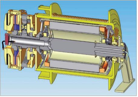
One significant benefit of PM motor over AC asynchronous motor is power density. Permanent magnet motors can produce as much as 30-40% more power density than a conventional and similar-sized AC asynchronous motor.
