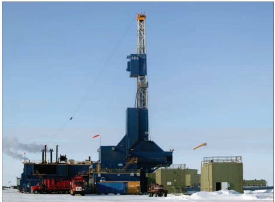
Nabors Alaska Rig 2-ES is working for BP on Prudhoe Bay, Alaska. Red Super Sucker trucks can be seen left of the rig vacuuming cuttings into the truck for disposal.
