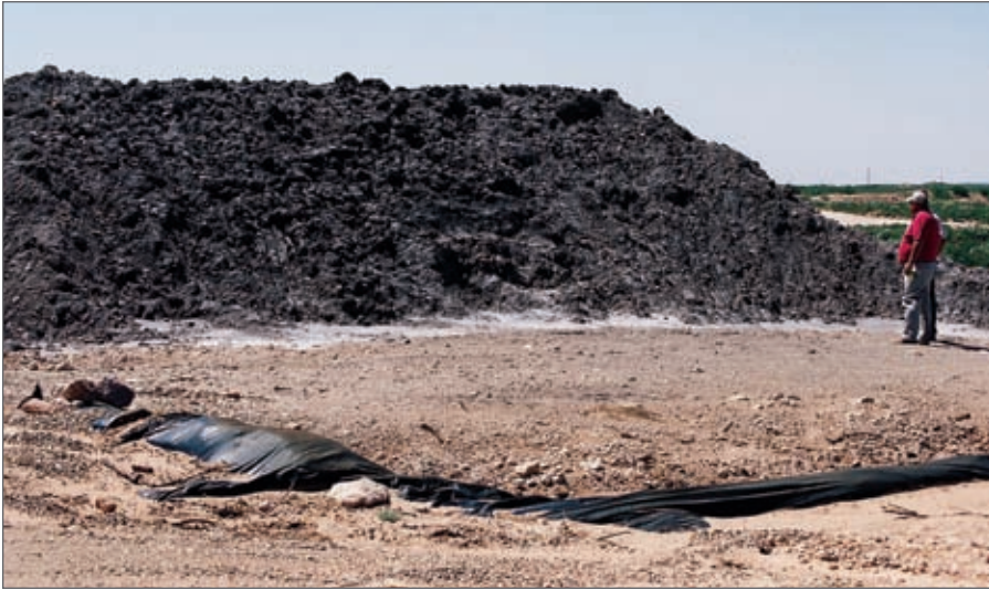
In the closed-loop system, dried cuttings are the only waste products generated. No significant amount of fluids is removed except contaminated mud and cement returns.
