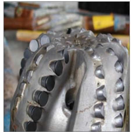
Figure 4: The mill was pulled in good condition after active parameter management to mitigate stick-slip and vibration (case study 3).
