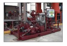
THE SECURE Drilling System is a closed-loop system that analyzes available drilling data to detect kicks or losses and automatically manages backpressure at the surface to control influxes
