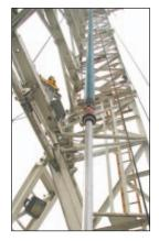
BAKER OIL TOOLS' linEXX Solid Expandable Monobore Liner Extension System optimizes casing configurations for drilling deeper or isolating trouble zones without reducing critical hole size. The system consists of the RC9 series casing shoe, FORMlock expandable liner hanger/packer, linEXX solid expandable casing, RNX retrievable guide shoe and catEXX hydraulic, top-down expansion system.
