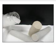
BAKER OIL TOOLS' Diamond FRAQ is the first VES fluid with polymeric fracturing fluid performance properties and superior formation and proppant pack cleanup capability. Its micelle stabilizers extend VES fluid use to 300° F. Viscosity enhancers reduce VES loading and total system cost. Fluid loss control agents significantly reduce fluid leak-off to at least 2,000 md and 250° F, to reduce fluid treatment volume and improve fracture geometry.
