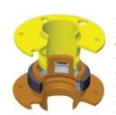
VETCO GRAY'S NEW marine riser system, the MR-6H SE, combines field-proven technology of the H-4 subsea wellhead connector and the dog-style marine riser (MR). To make the fully automated connection of the MR-6H SE, hydraulic units on the spider engage a cam ring on the box, which actuates 6 dogs into the profile in the pin. This creates a full pre-loaded connection with an efficient and effective load path.
