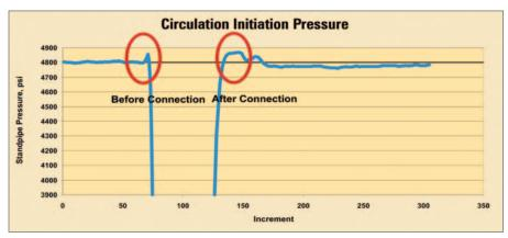
Above: With its constant, low-energy gel structure, pressure spikes associated with initiating circulation are virtually eliminated with the RHEO-LOGIC system. Below: Surge pressures when running casing with the RHEO-LOGIC system are reduced when compared with conventional SBM, resulting in minimized downhole mud losses.
