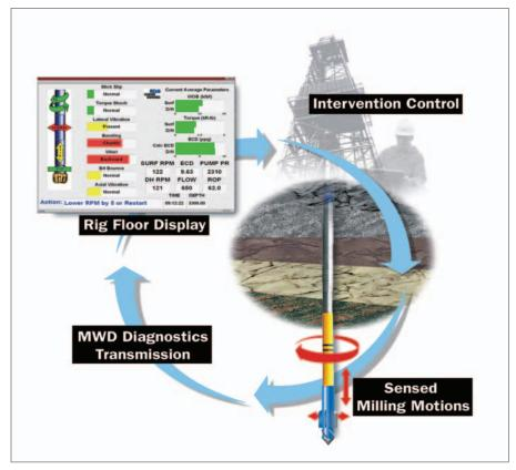
Baker Oil Tools' Smart Intervention system involves downhole data acquisition and processing in the Sentio sub; bi-directional data transmission to surface via MWD tools; and use of data for surface process control of intervention operations.
