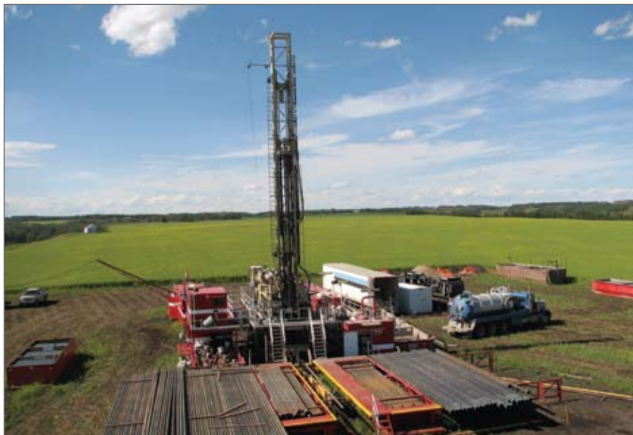
The Atlas Copco RD20, seen above on a gas well location in Alberta, Canada, has been used to drill pre-sets for larger rigs. Using a "mixed fleet" approach has the potential to help contractors save time and money.
