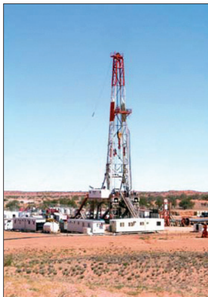
Figure 7: Century Drilling Rig #27 on location in Cooper Basin, Australia, for Geodynamics developing renewable geothermal energy. The operator drilled a vertical geothermal production well underbalanced into hot fractured granite at 14,000 ft, maintained pressure stability, minimized mud losses, preserved fracture permeability, controlled water kick and reduced mud weight 1.0 ppg using the DAPC system.
