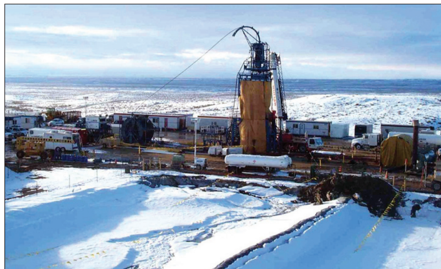
Figure 6: Coiled tubing rig drilling an underbalanced 14,000-ft MD directional well in Wyoming. The operator stabilized pressure to drill unconventional tight gas sand with constant BHP at 7,800 psi while continuously managing backpressure between 400 to 600 psi. Operator was able to identify micro-fracture system by monitoring backpressure fluctuations as small as 4 psi using the DAPC system.
