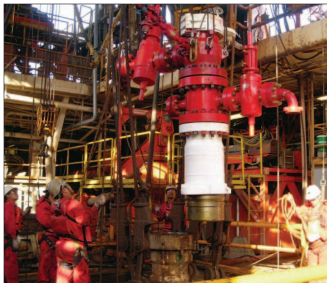
A PMCD rig-up on semisubmersible. The earliest MPD operations in Southeast Asia were from a semisubmersible rig.
