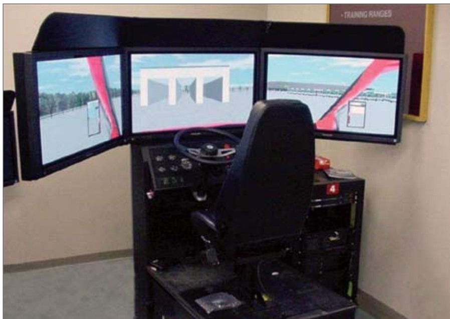
Simulators in the program featured high-tech graphics that allowed students to "drive" in three virtual worlds — off-road, rural/small town and large city — and in a variety of vehicles, including oilfield-specific frac pumps, N 2 tankers and bulk sand trailers.
