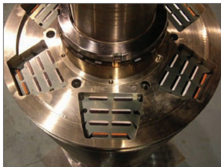
Above and below, GE's interior permanent magnet motor features an equivalent power rating of 1,500 hp. The cage of the rotor contains the magnets. This design approach results in improved constant power speed range compared with surface-mounted PM technology, according to GE.
