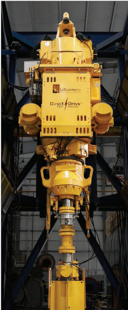
Above, LeTourneau Technologies' Direct Drive top drive uses a patented AC electric motor. LTI says it has done preliminary designs but has not built a PM motor yet.
