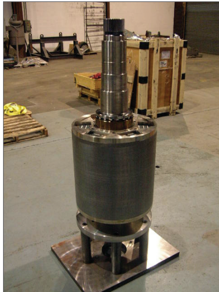
Above and below, GE's interior permanent magnet motor features an equivalent power rating of 1,500 hp. The cage of the rotor contains the magnets. This design approach results in improved constant power speed range compared with surface-mounted PM technology, according to GE.
