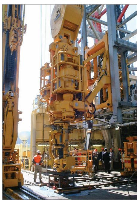
Hydralift, now a part of National Oilwell Varco, developed the Hydralift Power Swivel - 500 (HPS) in 1992. Soon, changes were made to include an integrated swivel, as well as critical design improvements in the upper gearcase sealing system, ultimately providing a more modular design.
