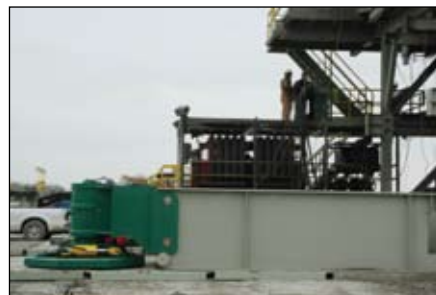
Veristic's Rig Walker allows drillings rigs to be moved laterally without rig-down.
