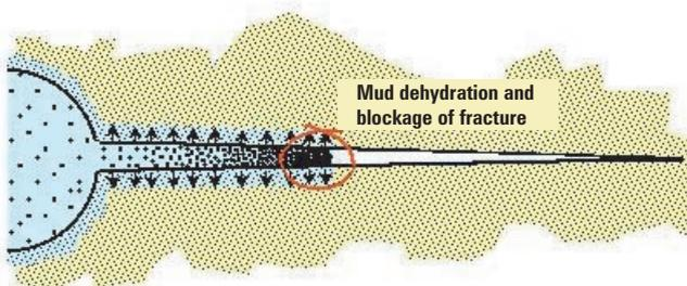
the proximity of older wells and fractured formations results in increased risks of severe uncontrollable losses.
