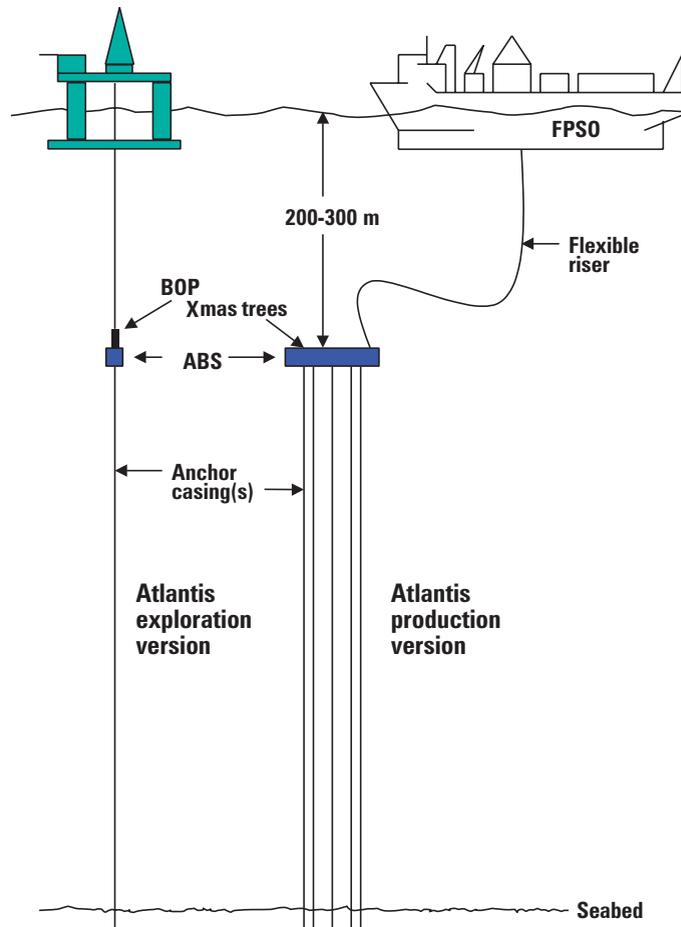
**Figure 2: Atlantis dual gradient drilling**
