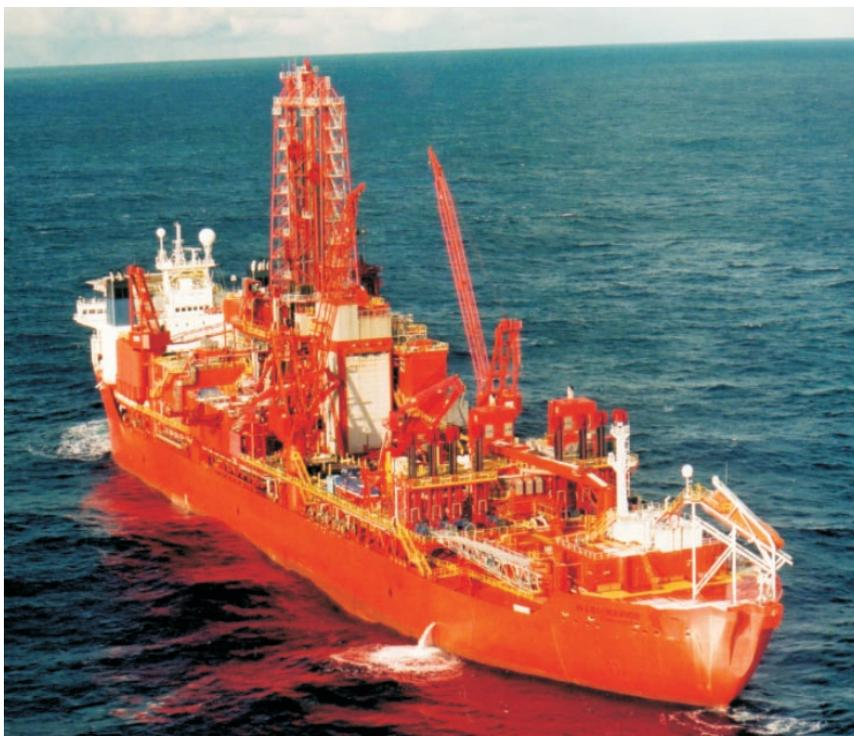
**Smedvig Offshore's West Navion drillship completed the Qullec-1 well offshore Greenland in about 80 days while facing challenges of remote location, deep water and iceberg management.**
