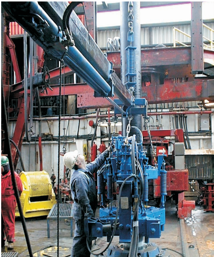
Leadhand provides a safe approach to manipulating a hydraulic power tong. Hydraulic power supply can be self-contained or drawn from existing rig supply.
